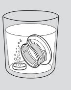
After cleaning it, replace the filter cap in the  $\mathfrak{a}$  position and turn it to the right, to the  $\mathfrak{a}$  position
